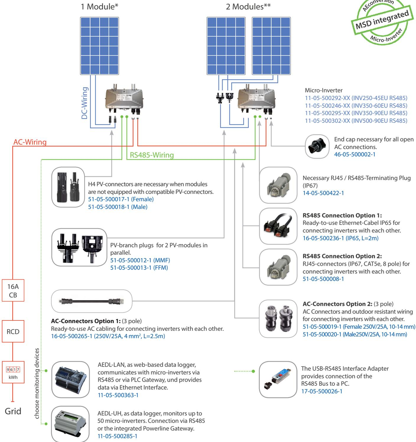
\* 1 Module: 45V, 60V or 90V max. depending on inverter version
